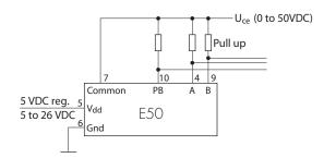
Because driver ULN2003A, equipped with "Open Collector Output" and integrated supression diodes for inductive loads is used, the cathodes of all diodes = Common (7) have to be connected to UCE. The pull-up resistors are also connected to UCE. This circuitry protects the encoder against e.g. surge currents.
