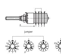
12 positions; the coding will be made according to the layout on the left.
