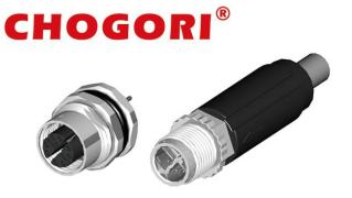
Designed and tested to achieve superior signal integrity, Chogori's M12 X-code connector series conforms to IEC 61076-2-109 standard. Its cross shielding design aims at eliminating crosstalk and unwanted signals during transmission. Fully (360°) shielded paired with Cat 6a cable, the M12 X-code assembly achieves Ethernet speed of up to 1/10 gigabits per second (Gbps) providing increased transmission rate and efficiency compared to
