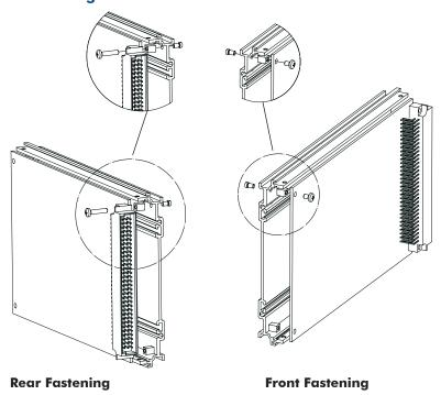
The PCB can be fastened to the front or rear of the side extrusions
