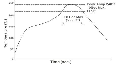
Note: The curve only applies to the hot air reflow soldering
