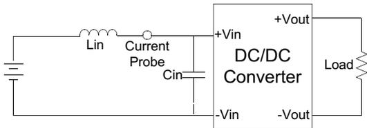
**Output Ripple & Noise Measurement Test**
