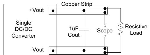
**Input Reflected Ripple Current Test Step**
