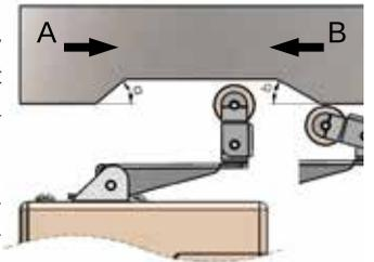
The limitations on the striking angles are the same as for an indirect roller lever, with a limitation on speed of 2 m/s.
