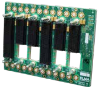
6-slot backplane enables high speed signal processing and PNT
