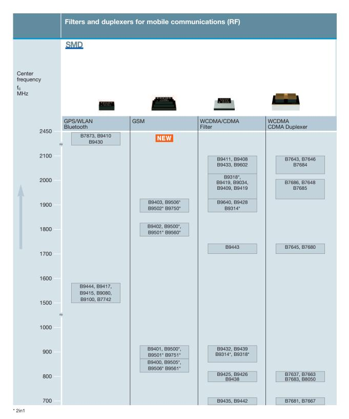
Surface acoustic wave components are electronic components in which piezoelectric effects are utilized to produce band-pass characteristics.
