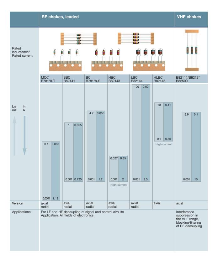
The proven RF and VHF chokes from EPCOS have outstanding RF and temperature properties as well as excellent saturation behavior.
