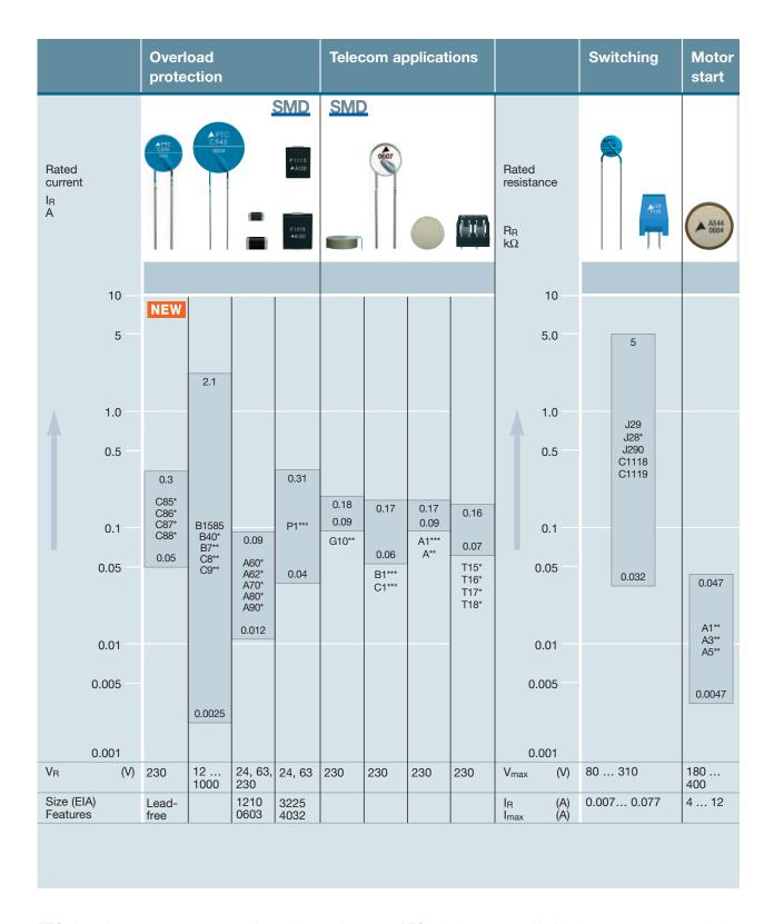
PTC thermistors are temperature-dependent resistors. They measure and control temperatures, protect against overload and serve as heating elements.
