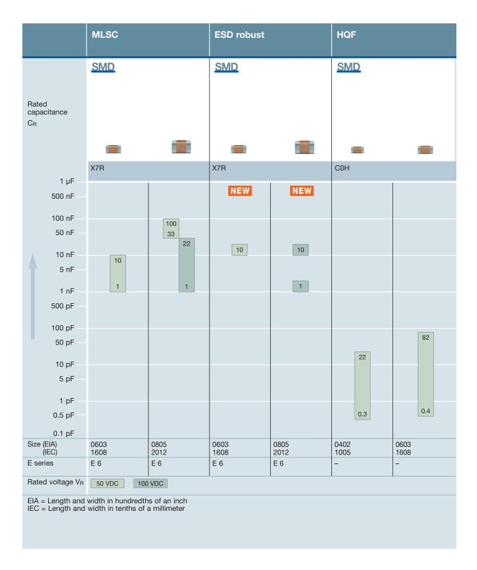
The MLSC series provides highest functional reliability while saving space on the board thanks to the integration of two series capacitors in a single component.
