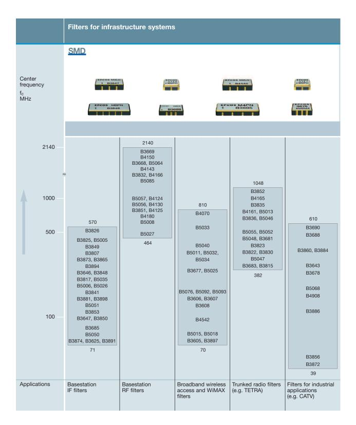
Surface acoustic wave filters play a key role in the infrastructure systems of modern telecommunications. Because of their special features, these products are increasingly being used in various infrastructure systems such as mobile phone base stations, wireless local loop and trunked radio systems, or cable TV networks.
