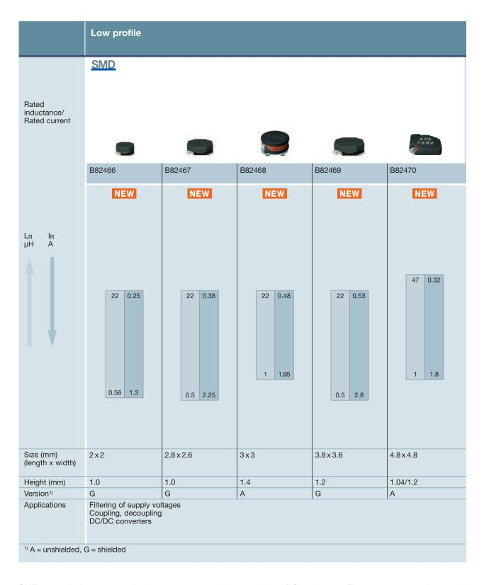
SMT power inductors extend the power range of the SIMID series towards even higher currents. The major characteristics of power inductors are high rated current
