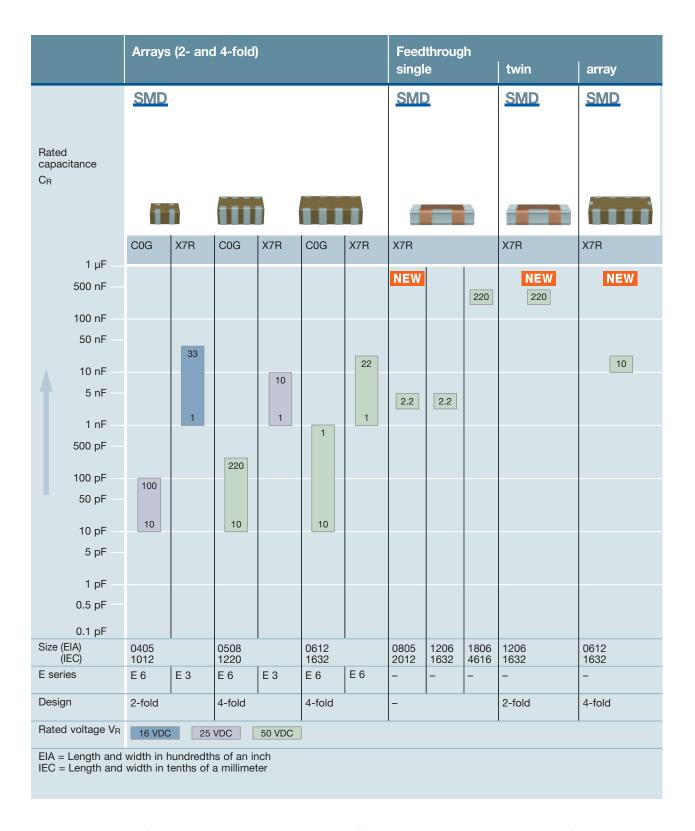
Arrays allow especially high placement and integration density on the PCB board. Thus they help cutting the cost and time for placement.
