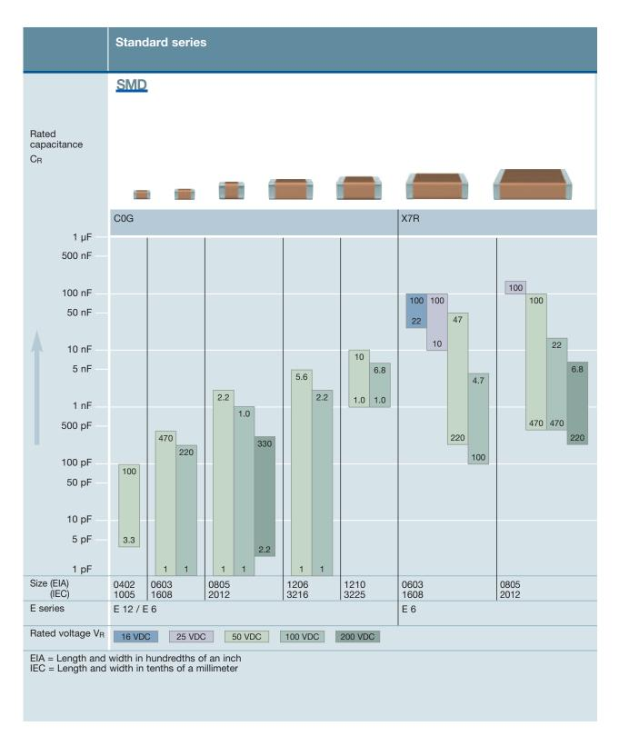
Multilayer ceramic capacitors (MLCC) offer maximum capacitance within the smallest space. They are needed in many areas of advanced microelectronics, for instance
