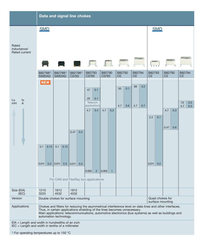
Data line chokes ensure electromagnetic compatibility (EMC) in the sector of data and signal transmission. They already suppress asymmetrical interference coupled onto
