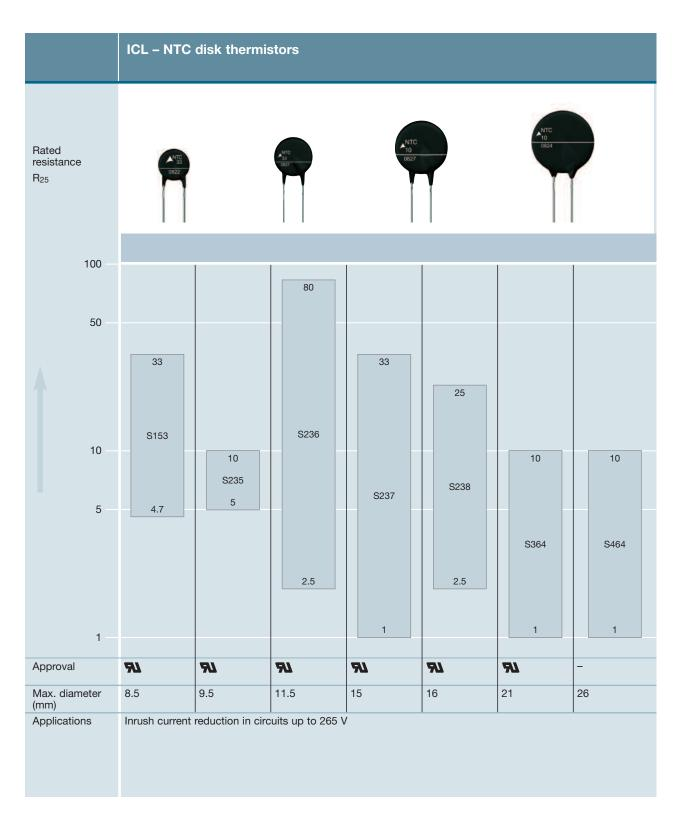
Many items of equipment like switch-mode power supplies, electric motors or transformers exhibit excessive inrush currents when they are turned on. The thermistor limits the current at turn-on by its relatively high cold resistance. As a result of the load current the thermistor heats up and reduces its resistance.
