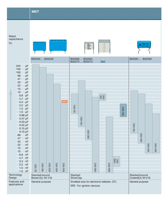
Metallized film capacitors have almost unlimited self-healing capability. Short circuits are thus largely nonexistent. They exhibit high pulse handling and ripple current capability together with long life time. Typical
