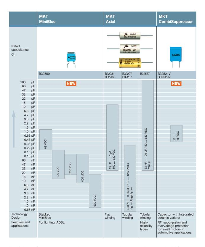
The MKT CombiSuppressor comprises a film capacitor and a multilayer ceramic varistor connected in parallel in a plastic case. This is a space-saving solution for EMI
