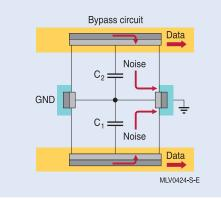
while the matched capacitances  $C_1$  and  $C_2$  (in this example 2 × 100 pF) of the MCVA provide effective EMI filtering of the bus data lines, especially for the frequency range 100 to 200 MHz.
