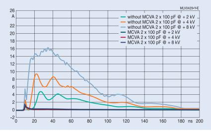
Besides the EMI/ESD protection (ESD protection level of >15 kV) an MCVA furthermore withstands load dump pulses up to 27 V/ 0.3 s as well as jump start pulses up to 28 V/ 60 s. This makes the MCVA a highly suitable component for automotive applications.
