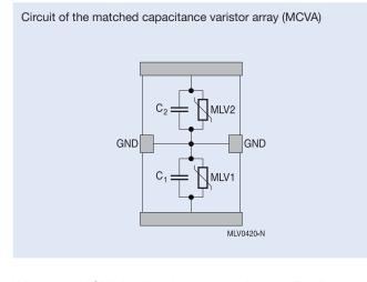
When the MCVA is directly integrated in the FlexRay termination (see figure 5), the ground capacitor  $C_s$  of the FlexRay termination is then in serial connection with each capacitance of the MCVA. Thus the ground capacitor reduces the parasitic capacitance to ground
