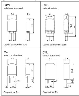
standard leads: Stranded wires 0,25 mmf00 or 300 mm length, Isolation Class B: colour yellow Isolation Class F and H: Colour white Stripped 5 mm
