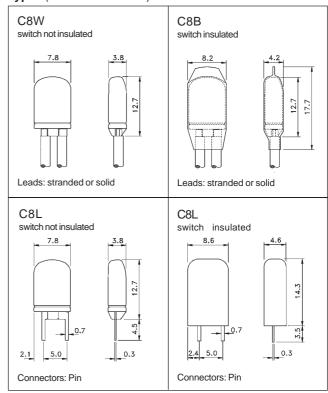
Standard leads: Stranded wires 0,50 mm²,100 or 300 mm long, Isolation Class B: colour yellow Isolation Class F and H: Colour white Stripped 5 mm
