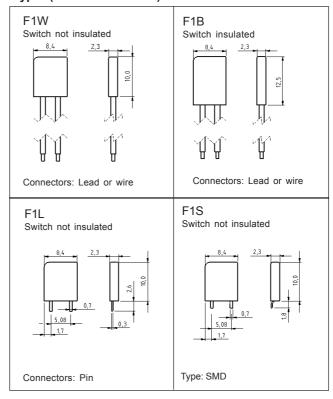
Standard leads: Stranded wires 0,25 mm², 100 resp. 300 mm length
