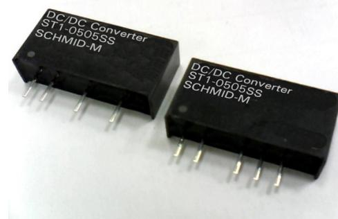
The ST1 series is a family of high operation temperature 1W single & dual output DC-DC converters. These converters achieve low cost, high efficiency, extra high temperature operation, continuous short circuit protection and SIP 7 pin size. Devices are encapsulated using flame retardant resin. The models operate from input voltage of 5, 12, 24 Vdc with output voltage of 5, 12, 15, ±5, ±12, ±15 Vdc.
