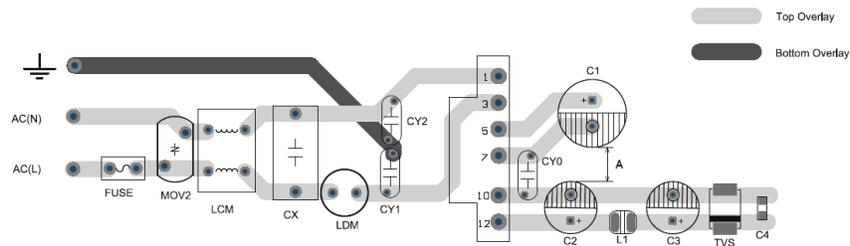
Figure 4: EMC application circuit PCB layout
