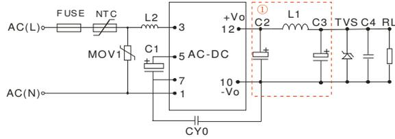
Figure 1: SLS03-R2S Typical application circuit
