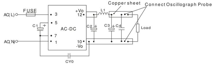
Note: CY0 is 1nF/400VAC Y1 capacitor, C1,C2,L1,C3,C4 refer to "EXTERNAL CIRCUIT PARAMETERS"
