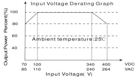
Note: When input 85~110VAC /240~264VAC/70~100VDC/340~400VDC, it need to be voltage derated on basis of temperature derating.
