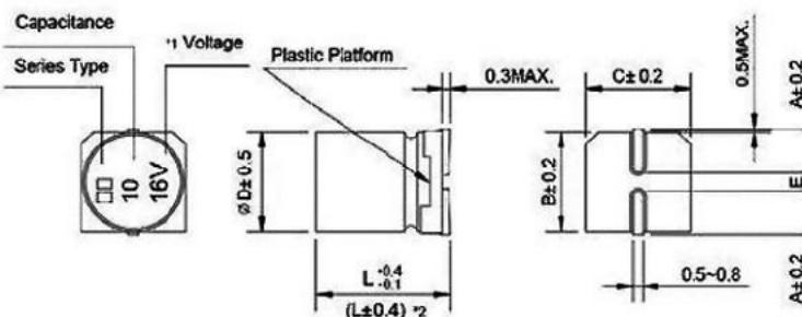
\*1 Voltage mark for 6.3V is [6V]      \*2 Applicable to Ø6.3\*7.7
